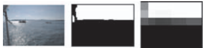
FIGURE 1 — Left: an image from our database with a blue-sky region; middle: a binary representation of the sky region’s coverage in the original image size; right: the downsampling of the binary image to 6 \times 8 pixels, which is used to perform PCA. The gray-scale values represent the relative coverage of the region at a given location: from 0% (black) to 100% (white).
