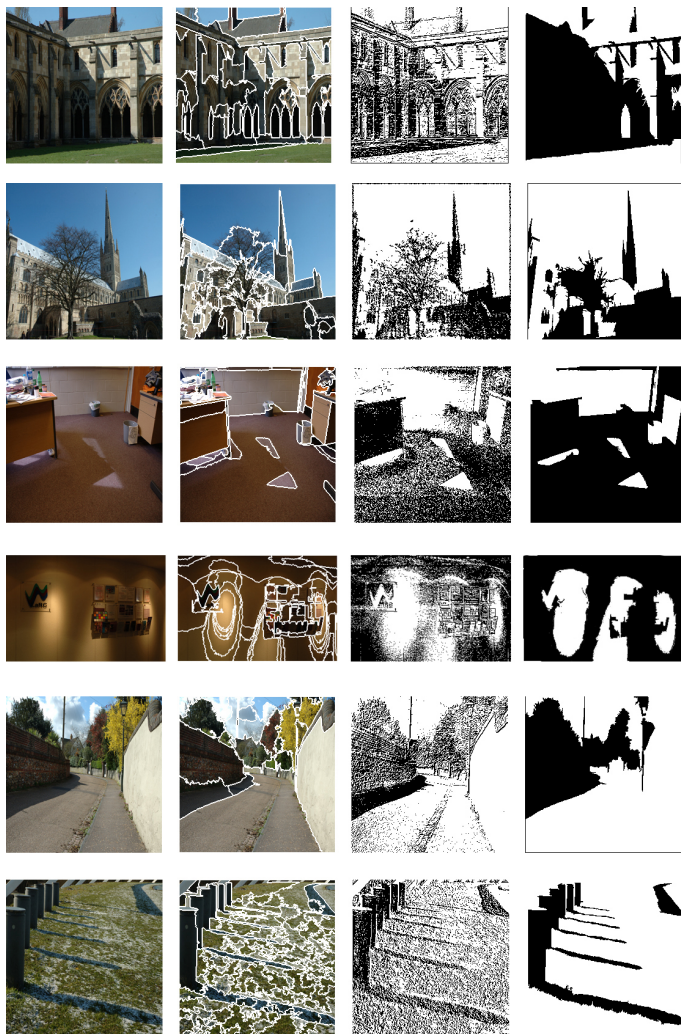
Fig. 8. Columns from left to right: the original images, the mean-shift segmentation; the region-based classification and the pixel-based classification.
