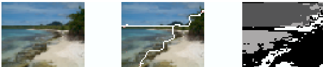
Fig. 2. An image segmented with edgeflow (middle) and DC Lab (right). Contrarily to Edgeflow, DC Lab regions, represented by different gray levels, are not spatially coherent.
