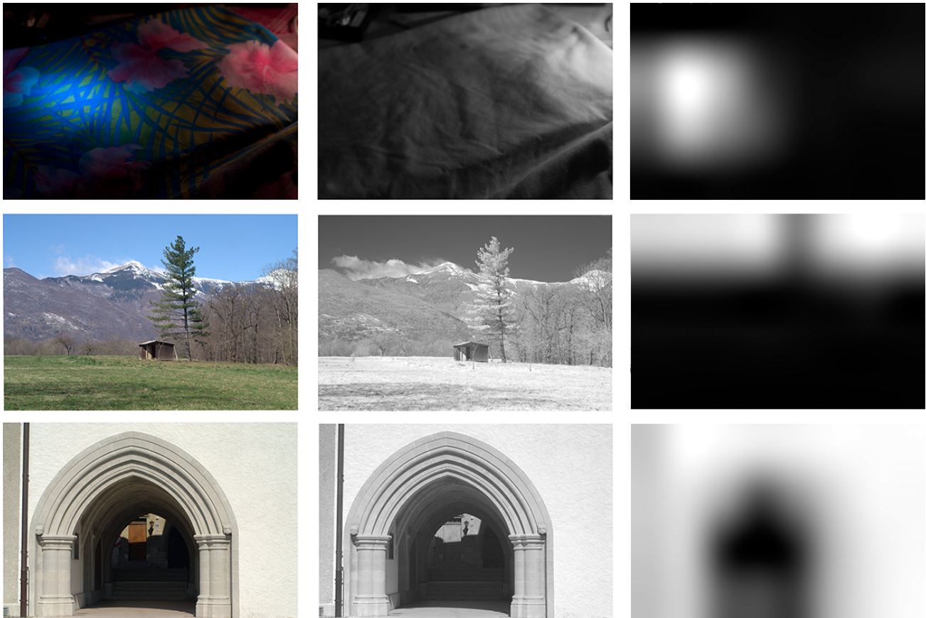
Figure 11. Column-wise: RGB image, NIR image, binary illuminant map. Top row: a cloth lit by an LED and a incandescent light bulb. Note how the bright and coherent LED light source disappears in the NIR. Middle row: a simple outdoor scene where the sky is very well detected from the rest of the sun-illuminated scene. Bottom row: outdoor shadow detection.
