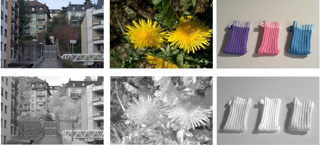
Figure 7. First and second row: RGB images and their corresponding NIR output. From left to right, the light conditions were: overcast sky, sunny day, incandescent lamp. The calculated colour temperature of the scenes were 7,500K, 5,000K, and 3,000K. The middle image is particularly interesting given that its lack of blue content make it very difficult for standard illuminant estimation techniques.
