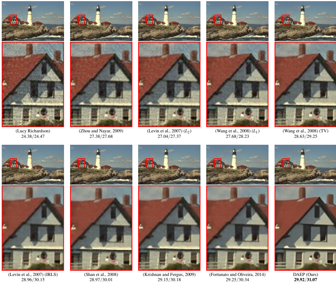
Figure 6: Comparison of non-blind deconvolution methods on the 21st image from the Kodak image set (Kodak, 2013). For each method, we report the PSNR ( dB ) of the visualized image (left) and the average PSNR on the whole set (right). The results of other methods were reproduced from Fortunato and Oliveira (Fortunato and Oliveira, 2014) for ease of comparison.
