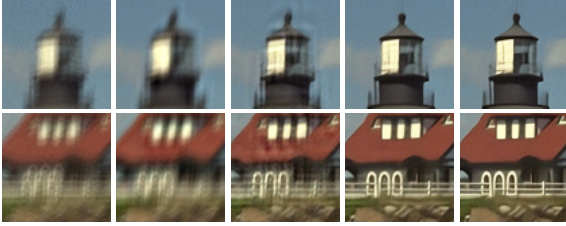
Figure 1: We propose a natural image prior based on a denoising autoencoder, and apply it to image restoration problems like non-blind deblurring. The output of an optimal denoising autoencoder is a local mean of the true natural image density, and the autoencoder error is a mean shift vector. We use the magnitude of the mean shift vector as the negative log likelihood of our prior. To restore an image from a known degradation, we use gradient descent to iteratively minimize the mean shift magnitude while respecting a data term. Hence, step-by-step we shift our solution closer to its local mean in the natural image distribution.
