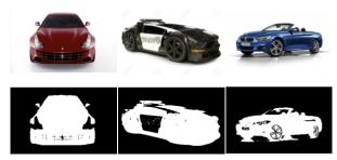
Figure 3: Sample images from  $\mathbf{W_{car}}$  and the corresponding segmentation masks generated from saliency combined with a dense CRF.
