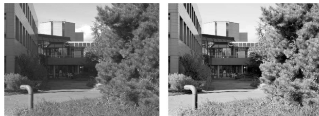
Fig. 1. Example of HDR scene that requires local processing. Left: Image rendered using a gamma correction. Right: Image rendered with the Retinex-based adaptive filter method proposed in this paper that combines global compression and local processing.
