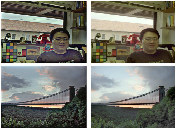
Fig. 9. Left: Image treated with MSRCR. Right: Image treated with the adaptive filter method. (Color version available online at http://ieeexplore.ieee.org .)
